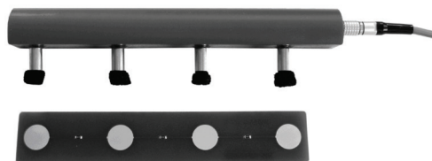
Fig 7.1 Wenner four-point probe with cable and control plate
